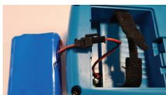
Then securely strap the battery back in place and re-secure the battery cover panel.
